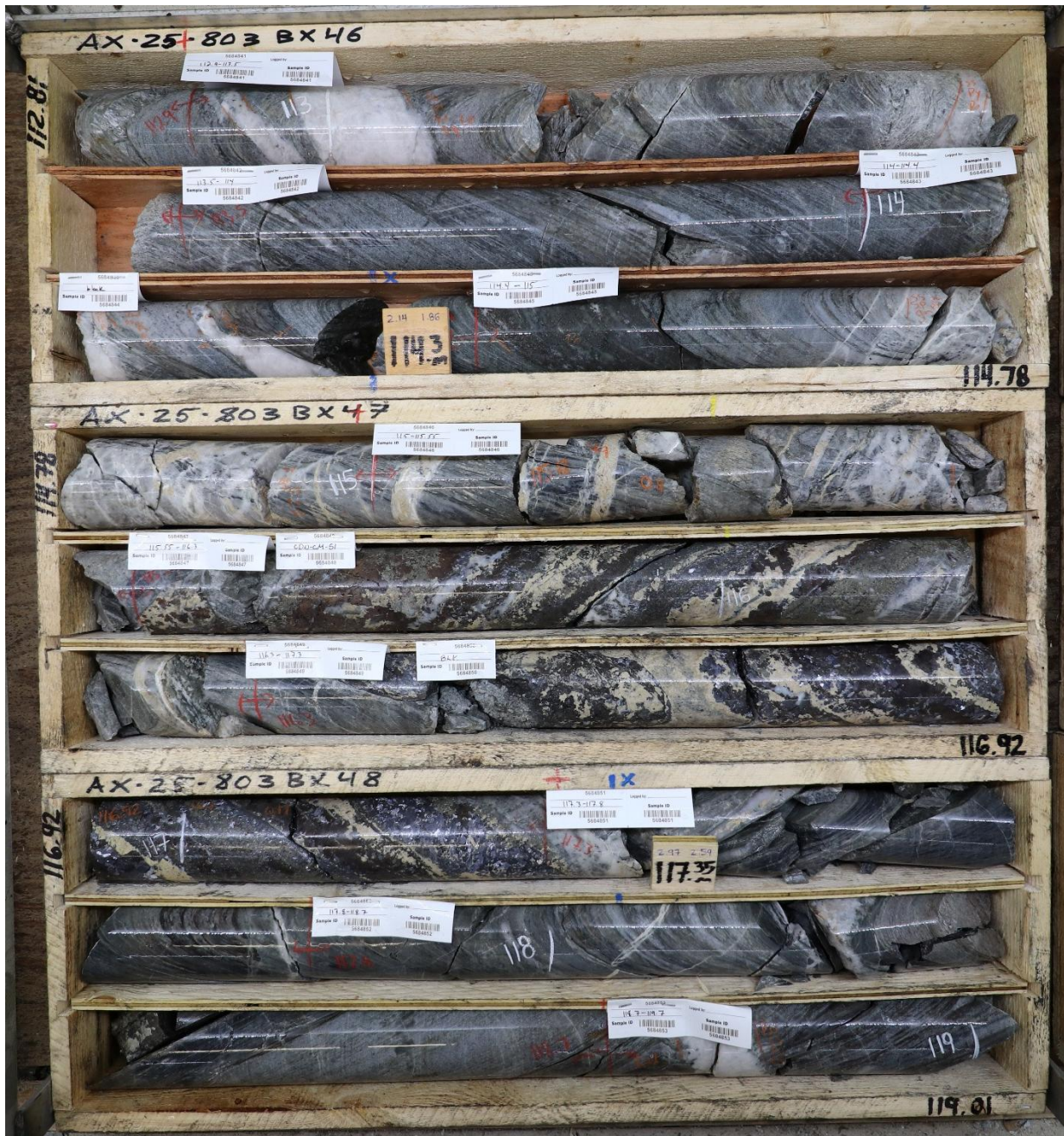
Figure 9: High-grade Keno-style mineralization in drillhole AX-25-803 in Ag-1 Vein in Powerline. Silver mineralization is associated with semi-massive galena and sphalerite mineralization hosted within discrete Fe-carbonate \pm quartz veins.
