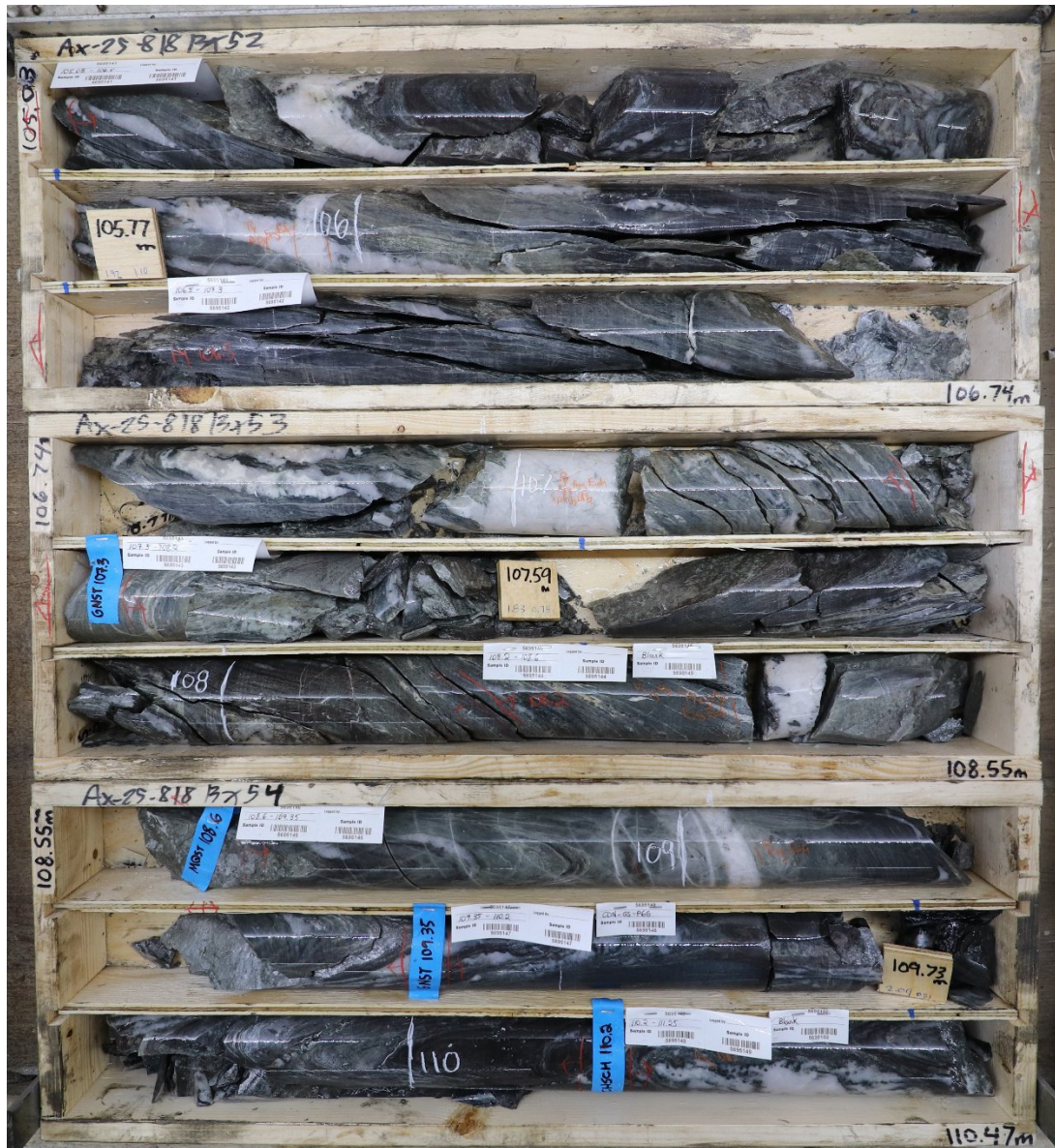
Figure 3: Diamond drill core from AX-25-818. Sheeted veins cutting metasedimentary rocks of the Hyland group, typical of the Powerline deposit hosting trace Bismuth sulphosalts, arsenopyrite and visible gold (See Figure 2).
