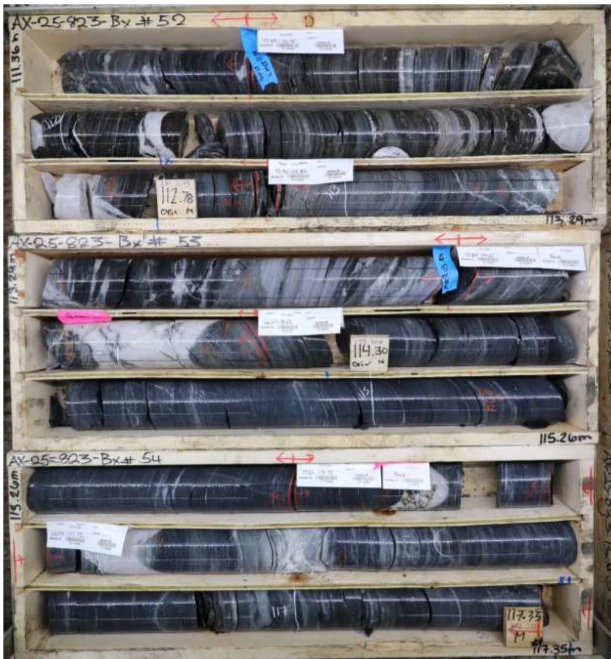
Figure 6: High-grade mineralization in AX-25-823 associated with sheeted quartz veins cross-cutting metasedimentary rocks of the Hyland Group. Sheeted veins contain visible gold grains intergrown with Bi-sulphosalts and arsenopyrite.
