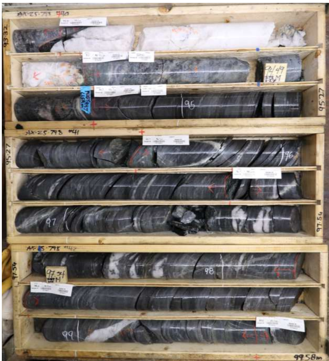
Figure 4: High-grade gold mineralization in AX-25-798 hosted in large cross-cutting quartz vein and associated centimetre-scale sheeted veins. Visible gold grains intergrown with Bi-sulphosalts in quartz veins are typical of high-grade mineralization in Powerline (See Figure 2).
