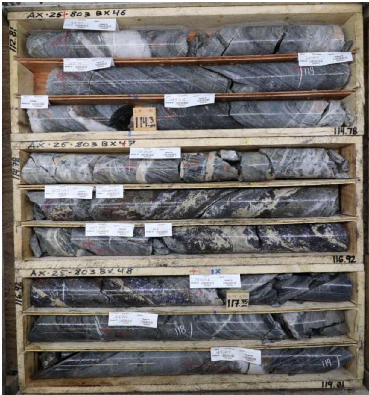
Figure 3: High-grade Keno-style mineralization in drillhole AX-25-803 in Ag-1 Vein in Powerline. Silver mineralization is associated with semi-massive galena and sphalerite mineralization hosted within discrete Fe-carbonate \pm quartz veins.
