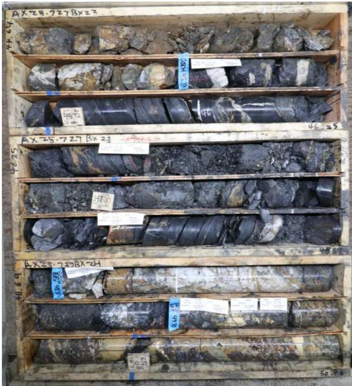
Figure 3: High-grade Keno Style mineralization in drillholes AX-25-727 in Airstrip. Silver mineralization is associated with galena and sphalerite mineralization hosted within discrete Fe-carbonate +/- quartz veins; in this interval, Keno mineralization is associated with brittle deformation concentrated at the contact between the Airstrip felsic dyke and Sourdough Hill Quartzite (Figure 2).
