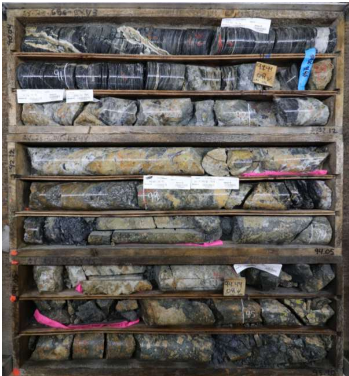
Figure 4: Brecciated Keno-style mineralization in an Fe-carb vein with galena and sphalerite in Airstrip from drillhole AX-25-686. Late brittle structures are the typical host for Keno mineralization at Aurmac.
