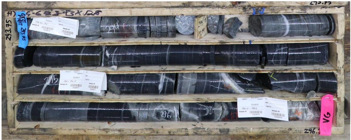
Figure 6: Sheeted (discordant) vein mineralization in footwall quartzites (below skarn mineralization) at Airstrip drill hole AX-25-678. Visible gold intersected at 296.3m. High-grade mineralization stratigraphically below typical “Airstrip-style” mineralization reinforces the potential for expansion at Airstrip and across the deposit.
