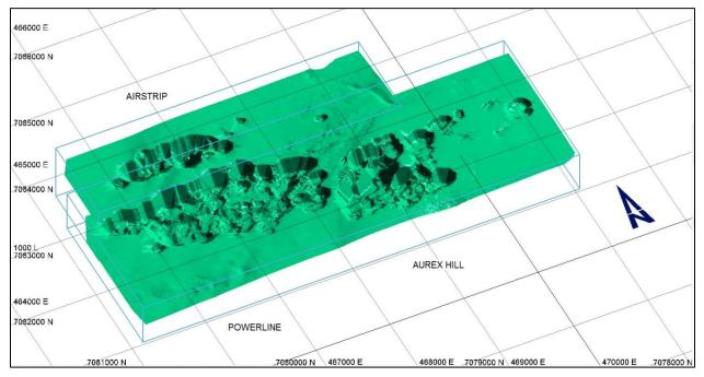
Figure 14-32: Mineral Resource Pits – Perspective View Looking Northeast – Airstrip, Powerline and Aurex Hill Deposits
