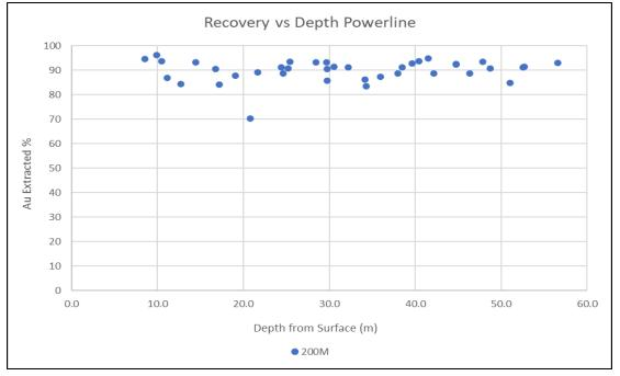
Figure 13-4: Recovery vs Sample Depth Powerline
