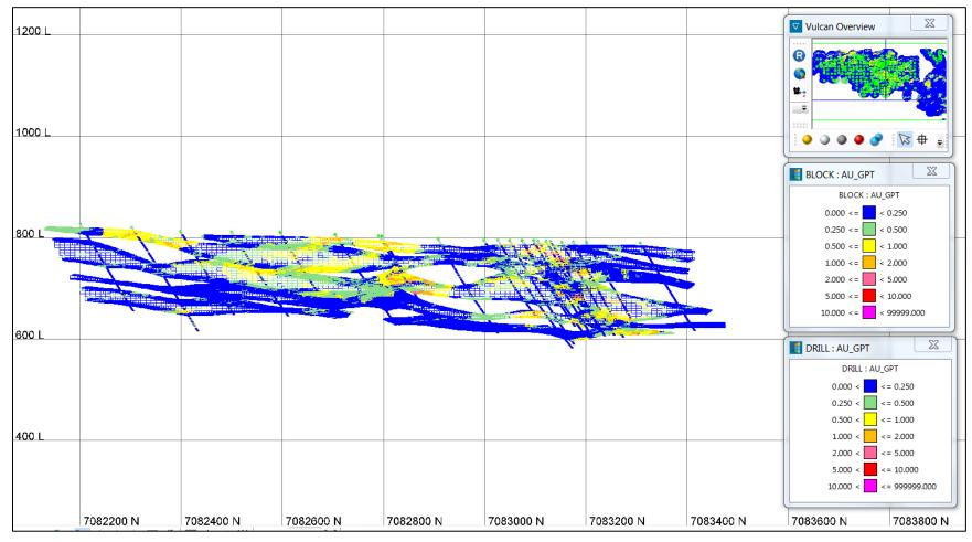
Figure 14-22: Gold Block Grade Estimates and Drill Hole Grades – Section 467,500E Looking West – Powerline Deposit
