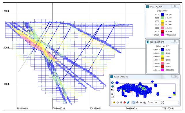
Figure 14-8: Gold Block Grade Estimates and Drill Hole Grades – Section 466,860E Looking East – Airstrip Deposit
