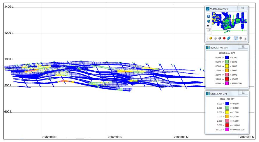
Figure 14-25: Gold Block Grade Estimates and Drill Hole Grades – Section 469,250E Looking West – Aurex Hill Deposit
