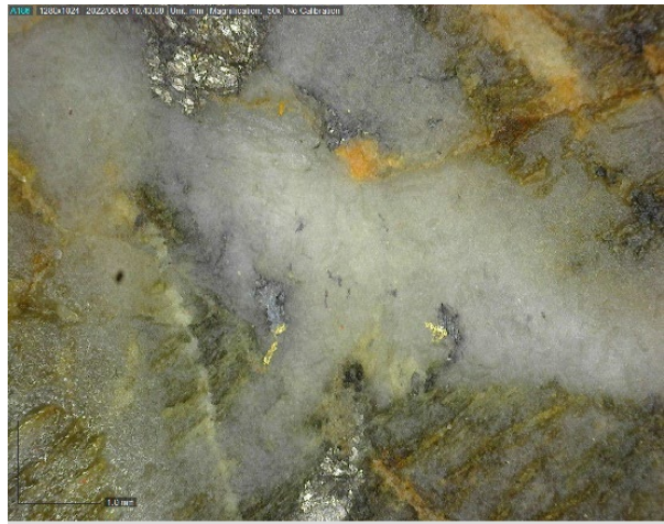
B) AX-22-337 61.6 m to 62.2 m 9.24 g/t Au over 0.6 m
