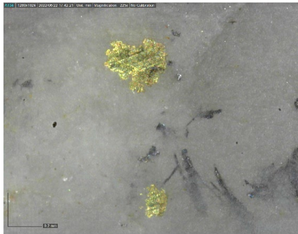
D) AX-22-293 70.1 m to 71.6 m 6.95 g/t Au over 1.53 m
