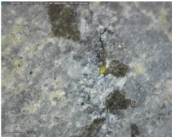
C) AX-22-327 26.7 m to 27.5 m 9.22 g/t Au over 0.8 m
