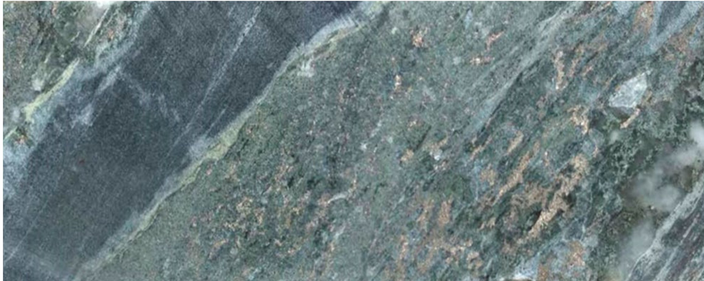
Actinolite-Chlorite-Quartz (Retrograde Skarn Alteration) carbonate replacement with disseminated pyrrhotite minor arsenopyrite and Chalcopyrite
